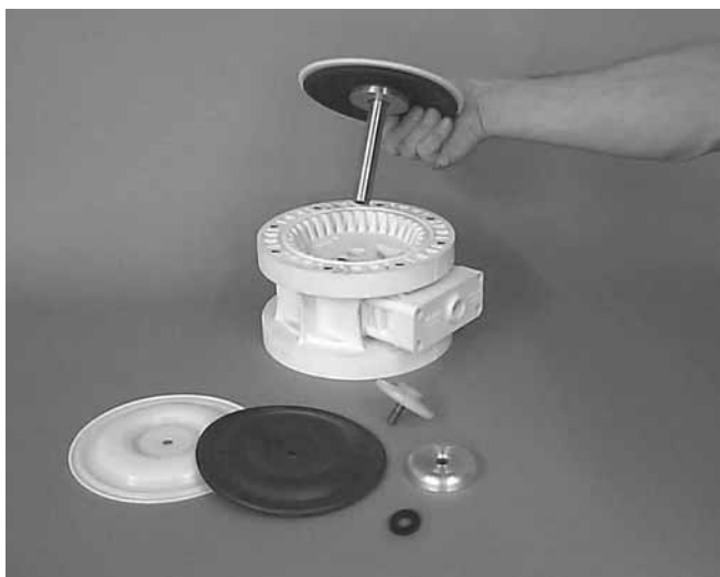
Step 10. Figure 10 After loosening and removing the outer piston the diaphragm assembly can be disassembled.
